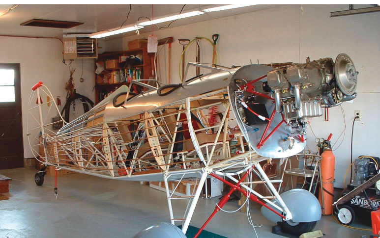
Thirty miles away, John welded the fuselage. They worked on installing the engine together.
