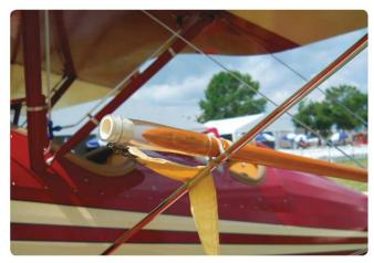
This owner uses a plastic cap to protect the point of his flying wire stabilizer, with a flag to remind him to remove it before flight.
