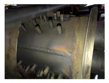
Example of crack in muffler (Image courtesy of Ben Showman)
