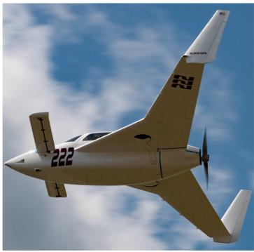
An interesting point regarding the turns... our canard airplanes actually generate a large amount of lift in a turn, which means that we don't loose as much energy in a sharp turn as more traditional airplanes. So, while most airplanes try to do a wider, low-G turn, we don't have to do that to the same extent. That wider turn means you're covering more distance... and distance equals time... so this is another advantage of our birds.
